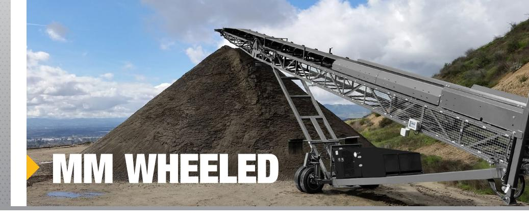
The MM80 and the MM100 Wheeled Stackers have been designed for high capacity stockpiling operations. All units come standard with diesel power units, hydraulic main lift and hydraulic top fold. Electric and dual power are both available as options based on the best application for the customer's business.
