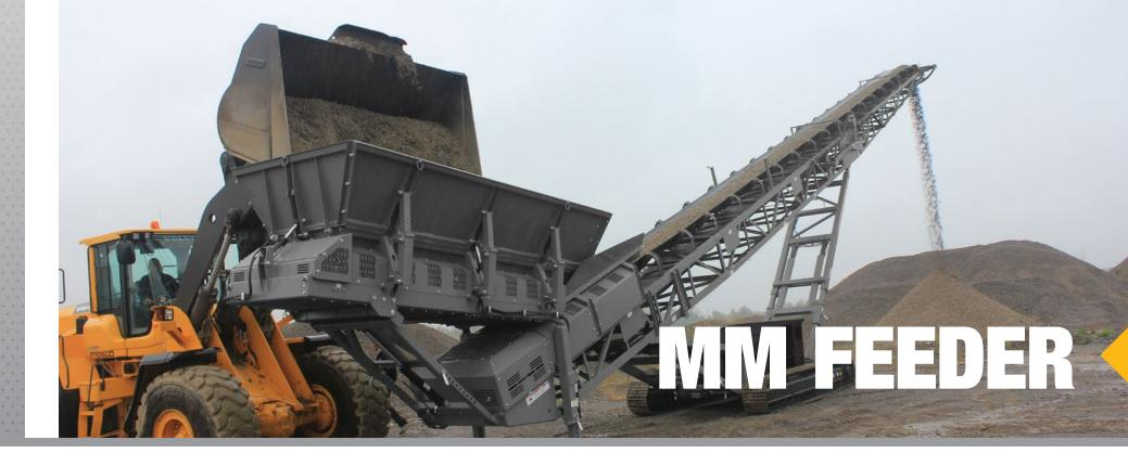
Material Mover's heavy duty high capacity feeder stackers, the MMF80 and MMF100, are designed to deliver enhanced handling and stockpiling of a wide range of materials across industries including aggregates, composting, landscaping and mining.
