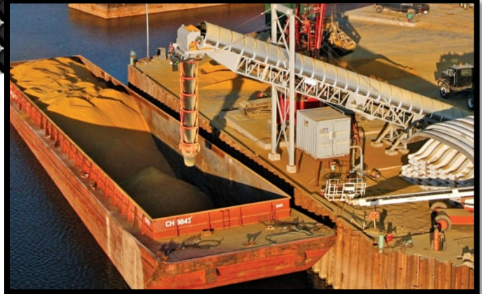
Barge Loading Conveyors
